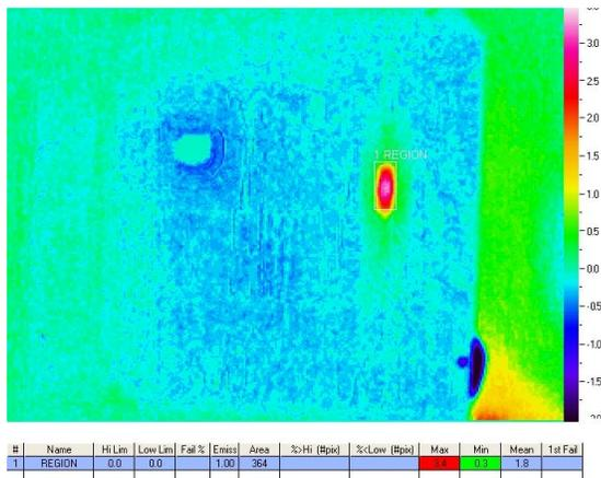
Fig. 3 Thermal picture highlighting the difference between a good and a faulty UUT. Fault location clearly shown.
