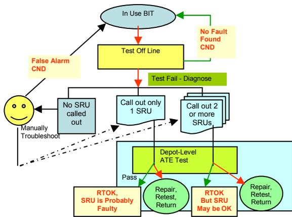
Fig. 1. CND and RTOK events in the Field and in Depot-Level ATE Test
