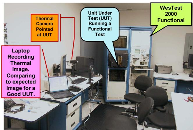
Fig. 2 Set up showing a thermal imaging integrated with an ATE running the test of a UUT.
